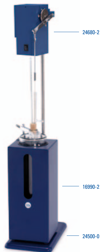
Typical Freezing Point setup
