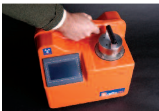
FIGURE 1 Monochromatic WD XRF per ASTM D 7039
