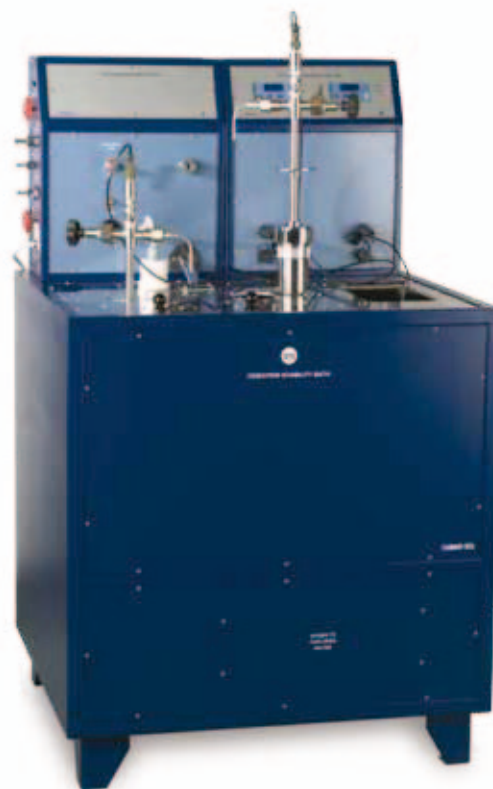
15400-4 with a 15450-3 Control Unit and two 15802-0 Oxidation Vessels installed
